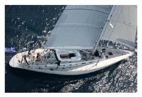
The hatches, fittings, and genoa tracks are flush into the teak deck, so that the spacious deck areas can be used for entertainment in the shade of a Bimini when riding at anchor, or for sunbathing while cruising under power at up to 10 knots with the 225 hp engine.
