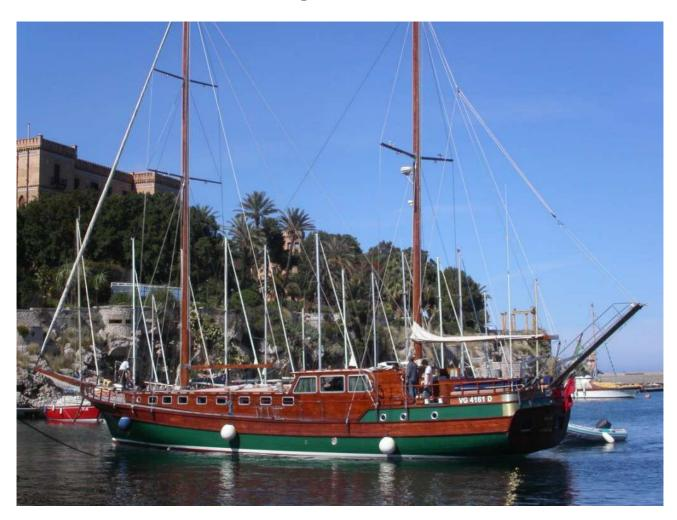
Flag Italy Year of Construction 1997 / 2005 24.00 mt. Loa Beam 6.10 mt. Draft 2.60 mt. Rigging Ketch Displacement 89 t. Hull Mahogany **Engine Cummins** 320 hp 9 knots (cruise); 12 knots max Speed Generator in all spaces Air conditioned Depth sounder, Radar, VHF, GPS, Equipment:
